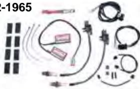
**Automatic Tune Kit** for all HD PC-V Power Commanders plugs directly into the PC-V with a single cable. It includes power connector that plugs into a bike’s harness. Rider can specify what air/fuel ratio to make each RPM and throttle position combination. Base settings are included and fully adjustable. Fits 1996-99 FLT.
