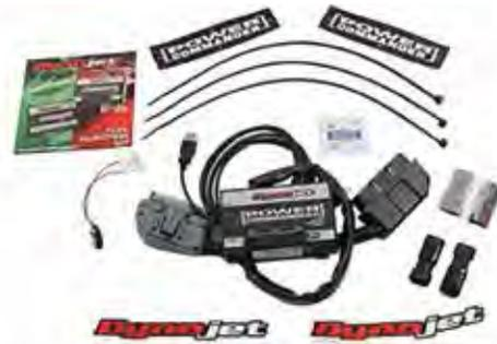
**Power Commander III USB Engine Management Systems** are for fuel injected models and allow for both fuel and ignition adjustments. Each unit includes a specific map, designed to improve performance over stock. The Power Commander includes IBM compatible link cable and software package which allows you to fully map the fuel ignition curves on IBM compatible computers. If a computer is not available, the fuel curves can be adjusted by using three touch buttons on the face plate.
