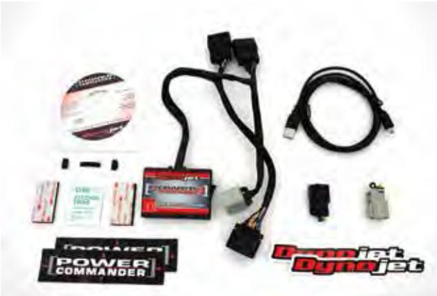
**EFI POWER COMMANDER V** features 2 position map switching function, gear and analog input. Power Commander V also allows each cylinder to be mapped individually and for each gear. This has 10 throttle position columns, and enhanced accel pump utility. Unit has a -100/+250 percent fuel change range and is compatible with 2009 and newer models. Fits 2014-16
