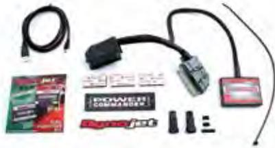
**Power Commander V Fuel and Ignition Timing Control** for each cylinder in a new smaller enclosure. Rev Xtend feature increases stock rev limiter. Switch between two maps “sent on the fly” can be adjusted on a “per gear” basis and allows for one map per cylinder per gear if required. Adjustment of fuel and timing is based on engine temperature provided by the cold start feature. Will power up with USB cable only for programming. **Note:** Not legal for use on pollution controlled vehicles.
