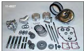
S&S TC-88 Cam, Carburetor, Pushrod and Piston Hot Setup Kit include Super "E" carburetor, adjustable pushrod set, pushrod covers, 570G cam (.570 lift), cam gear drive set and gear cover gasket kit. Installation of kit requires stock bore cylinders to be bored out to 3 7/8" and will increase compression ratio to 9.7:1 with stock cylinder heads. Order piston kit separately. VT No. 11-0027
