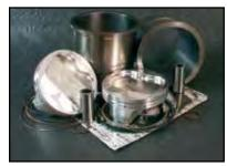
**1320cc Big Bore Kit** for V-Rod includes 12:1 compression forged Wiseco Piston Set with rings and matched 4.250 bore gaskets and sleeve set. Case boring required.
