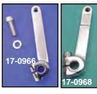
Chrome Steel Inner Shifter Lever Includes stainless allen screw and washer.
