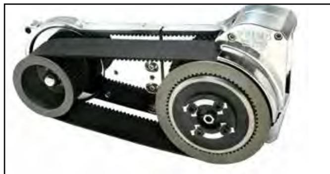
**Primo Brute V 14mm x 3 1/2 inch wide open "Super Street" Belt Drive.** Features diaphragm clutch spring that eliminates spring adjustment while distributing pressure evenly across clutch pak, motor plate, starter housing, hardware and outer guard. **\*Note** Can only be use with 1990-up starter.
