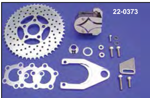
Edart Caliper-Disc Set includes 2 piston chrome billet caliper, polished rotor/sprocket combination with 49 teeth for 1" or 3/4" axle. Order bolt kit separately.
