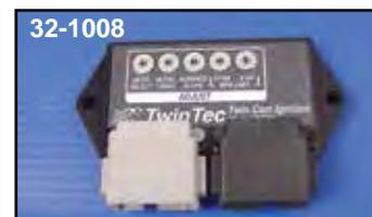
**Twin Tec External Ignition for 1999-06 Carbureted Twin Cam Models.** Wide timing advance adjustment range accommodates stock to highly modified engines. Features digitally set RPM Limit (100 RPM Steps). Selectable multi-spark mode for quick starting and smooth cruise. Coil outputs protected against short circuits. Billet aluminum housing with black anodized finish. Easy plug-in installation supports all sensors including theft/security module.
