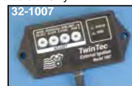
**Twin Tec External Plug In Ignition for 1990-99 Evolution Big Twins** features 4 rotary switches used to set the operating modes such as single or dual fire, adjust the timing, advance and select RPM limit. Two diagnostic LED's indicate status and start of the VOES switch. The status LED is also used for static timing as it will flash when the engine reaches top dead center.
