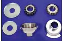
Chrome Mega-Neck Cup Set features 1" inner diameter bearing set with large outside diameter on the outer race which provides 1.68 times the radial capacity and 1.57 times the axial capacity of a conventional bearing. Kit includes chrome cups, bearings, races and two dust shields.
