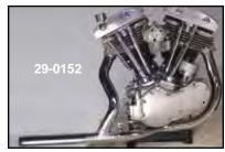
**Two Into One Exhaust** for rigid or swing arm frames on 1966-69. It is a three piece set incorporating the Y-flat pipe combination. Chrome **VT No. 29-0152**
