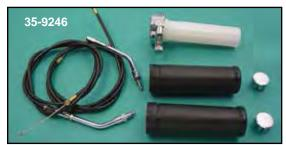
**Throttle and Cable Kits** include grips, throttle idle and Barnett throttle cable with ends attached as pictured for S&S 'E' and 'G' carburetors.
