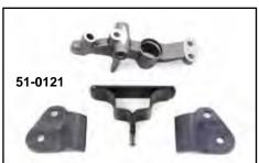
**Mounts for Bob Tanks.** "Our Original Frame Saver Kit" may be welded to all 1936-84 Big Twin frames, stock or custom, to replace original brackets.
