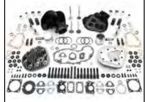
45" Top End Kit includes 45 valve cover kit, 45 lifter kit, valve spring kit, front & rear 45 cylinder, 2 Sifton intake valves, 2 Sifton exhaust valves, high compression head, gasket kit, headbolt kit. and washer kit.
