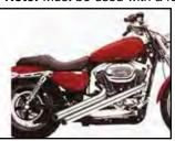
Chrome Vance & Hines Side Shots feature power chamber design, 2½" header pipe, 220° full length heat shields and removable baffles. Mounting hardware included. Fits 2004-2006 XL.
