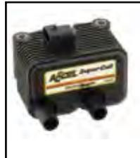
**Accel Late Model Super Coil** for late model Twins with carb. Features faster rise time, higher voltage, maximum spark and energy to spark plugs for quicker starting, improved idle and crisper throttle response. Fits in OEM location and is available in black finish. Fits 2005-06 All XL models.
