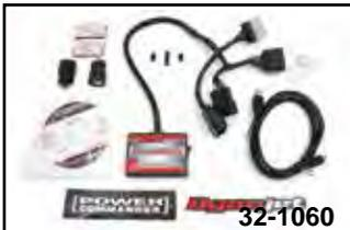
**Power Commander V** features 2 position map switching function, gear and analog input. Power commander also allows each cylinder to be mapped individually and for each gear. This has 10 throttle position columns, and enhanced accel pump utility. Unit has a -100/+250 percent fuel change range and is compatible with 2009 and newer models.
