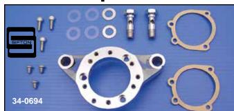
XL Billet Chrome Integral Breather/Carburetor Mount Bracket includes mount bolts for installation of any 3 bolt CV type air cleaner or velocity stack to be installed in vertical or horizontal position.
