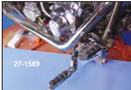
Chrome Footpeg 4" Extension places peg position on FXST 3 1/4" wider and 2" forward. Shown installed on 22-1001 forward controls. VT No. 27-1589
