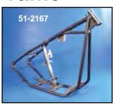
Big Twin Custom Rigid Frames. Straight leg style rigid frame for 4 or 5-Speed with or without bobbed mounts. Features 2½ stretch in front down tubes and 35° rake. Stock is 30°. Stock type neck accepts Wide Glide trees. Evolution style accepts flat side tanks, Shovelhead style accepts 1936-
