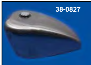
Bobber Gas Tanks are 2.4 gallon and feature 4 bolt mount strap system to be welded on to frame. Use mount kit 38-0214 included with tanks.
