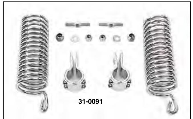
**Chrome Seat Spring Kit** is for use with stock seat "T" on rigid frame models. Kit includes a set of two 7" seat springs with loop mounts for lower studs, a three piece 1" I.D. clamp set, seat stud set, spring stud set, nylock nuts and flat washers. Fits 1936-1952 EL, 1941-57 FL.
