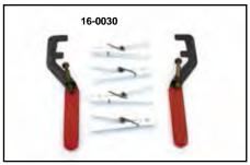
Crane Cams Installation Tool comes with easy instructions for the mechanic to install Crane's adjustable pushrods without removing the gas tank or rocker covers. In all FL-FX with adjustable pushrods, the tool makes it easy for cam changes. No removal of pushrods, pushrod covers, tappets or tappet guides. Tappets never have to fall out of the guides while doing cam changes.
