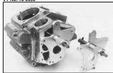
Cam Clearance Cutter bolts to 1970-up Big Twin cases and features an adjustable cutter and threaded depth feed. Power by ½" drill or use in milling machine. VT No. 16-0879
