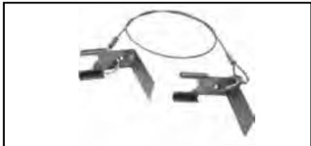
**Jims Beta Engine Hydraulic Balancer Retainer Tool** use these retainers to hold the hydraulic tensioners in place when repairing all Beta engines. The hydraulic tensioners are used to keep constant chain tension on the counter balancer system. Without the use of these retaining tools you will not be able to remove or install the balancing system. Use on all Beta Twin Cam engines 2000-up.
