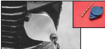
**Exhaust Stud Drill Fixture** fits 1984-up Ex Big Twin and XL ports to align for drilling of broken exhaust stud.
