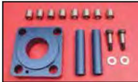
**Cylinder Jig Assembly** use to repair stripped damaged cylinder base threads up to a 4" bore, in engine case. This will hold centerline
